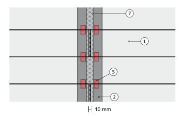
• To prevent the shifting of the profile in a horizontal direction, we recommend securing the profile nearest to the center of the length of the profile through a screw into the base joist so that the screw is covered with the following profile. At the junction of the profiles we recommend protecting the wooden base joists with bitumen or EPDM tape (7).
