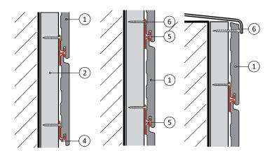
• The connection of the profiles is performed with two base joists side by side or one wider joist and two rows of standard clips. The maximum allowable overhang of the profile through the joist is 50 mm. To achieve a nice appearance, we recommend placing the connecting profiles alternately, thus in order to avoid a long vertical space.
